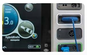
The active slot and the instrument in use are shown on the display and through the illuminated socket frame.
